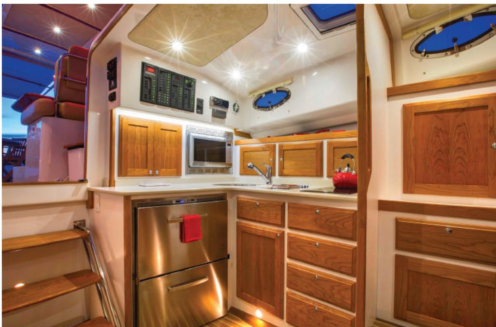
At the base of the companionway—at close proximity to the helm—is a galley with microwave oven, deep stainless sink, cooktop stove, and pull-out refrigerator/freezer.
